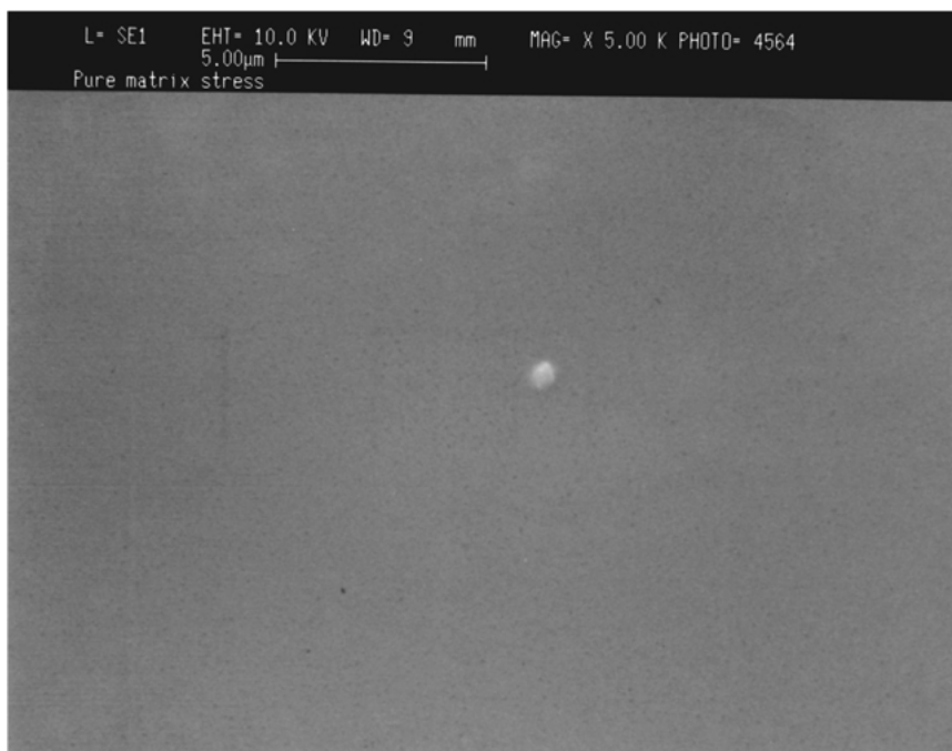
Figure 3 Fracture surface of unfilled rubber, no structure is noticeable in the cured sample (5,000 \times ).
